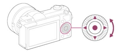
You can select setting items by turning or pressing the top/bottom/right/left side of the control wheel. Your selection is determined when you press on the center of the control wheel.
